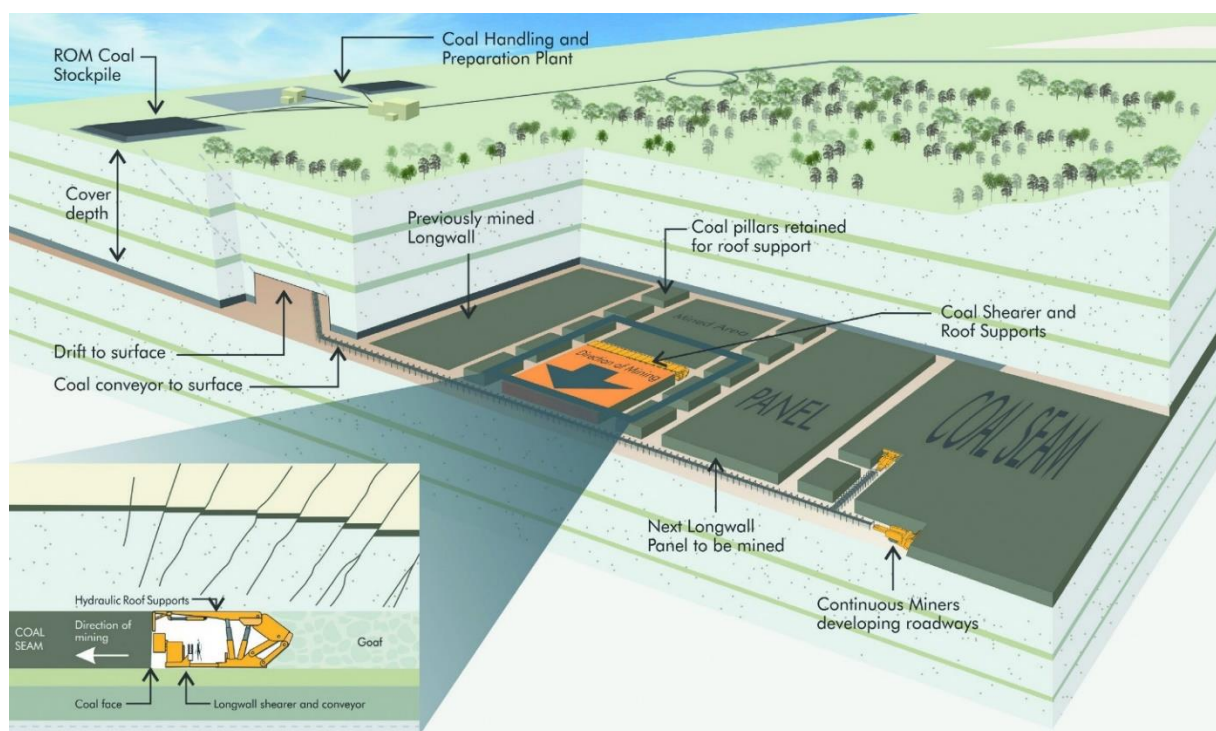
Figure 3.36: Longwall Mining Method Schematic
