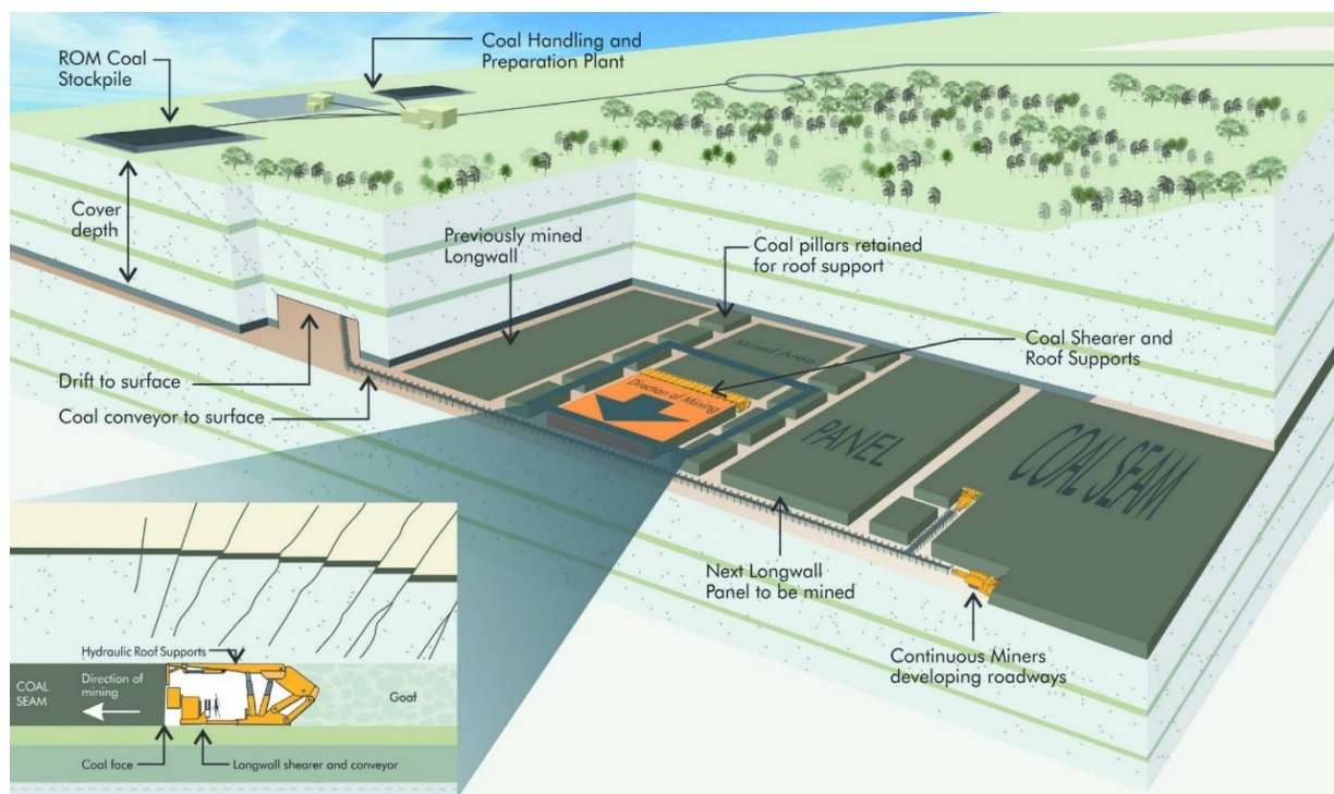
Figure 3.36: Longwall Mining Method Schematic
