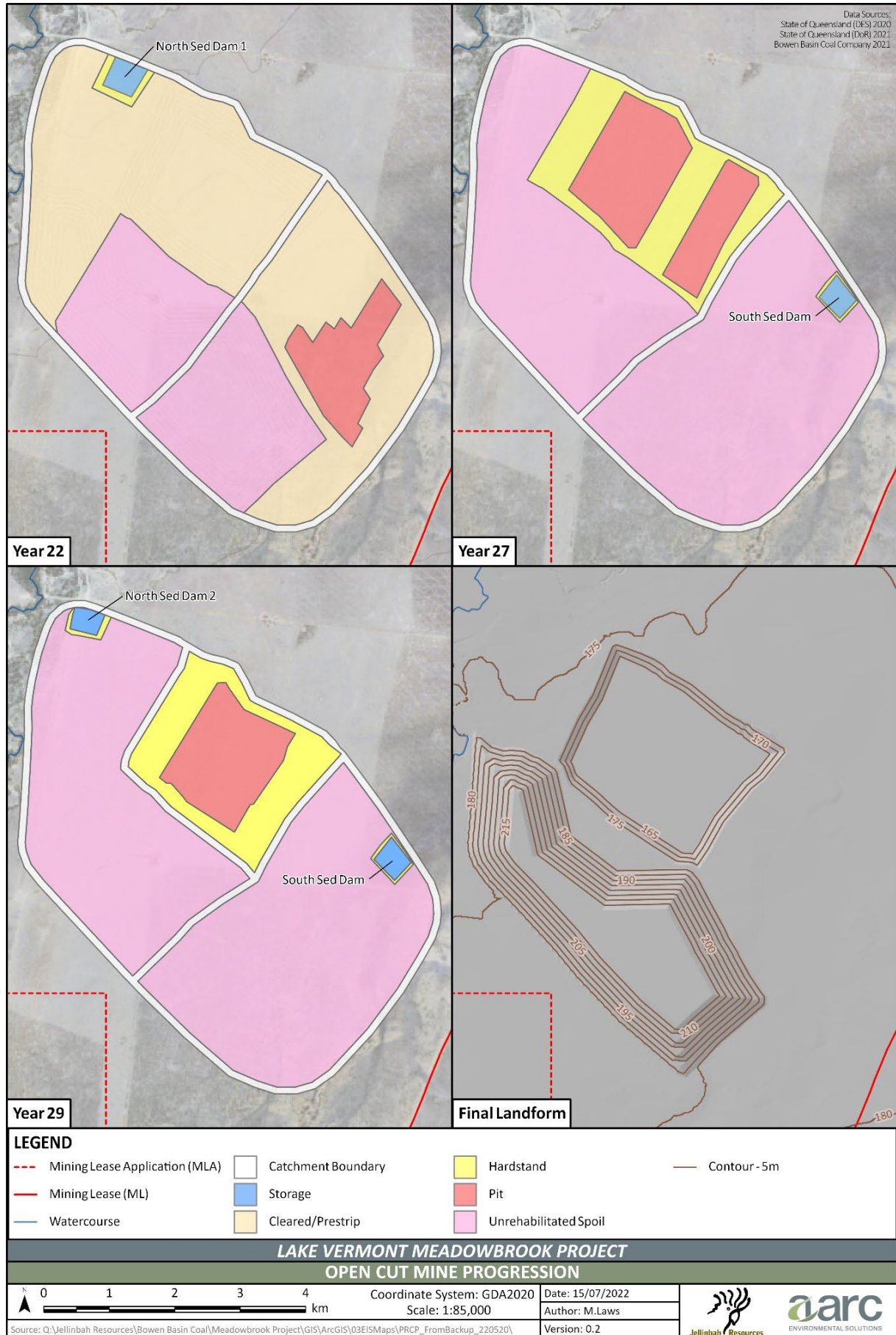
Figure 3.27: Indicative mine progression plan—open-cut pit mining
