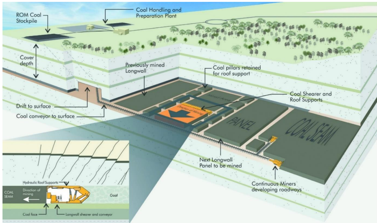
Figure 21.30: Longwall mining schematic
