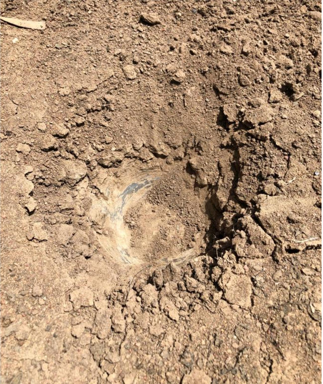
**Photo 4:** Attempted Hand Auger. Note compaction of clay on the bottom/edges of the bore – resulting in auger refusal
