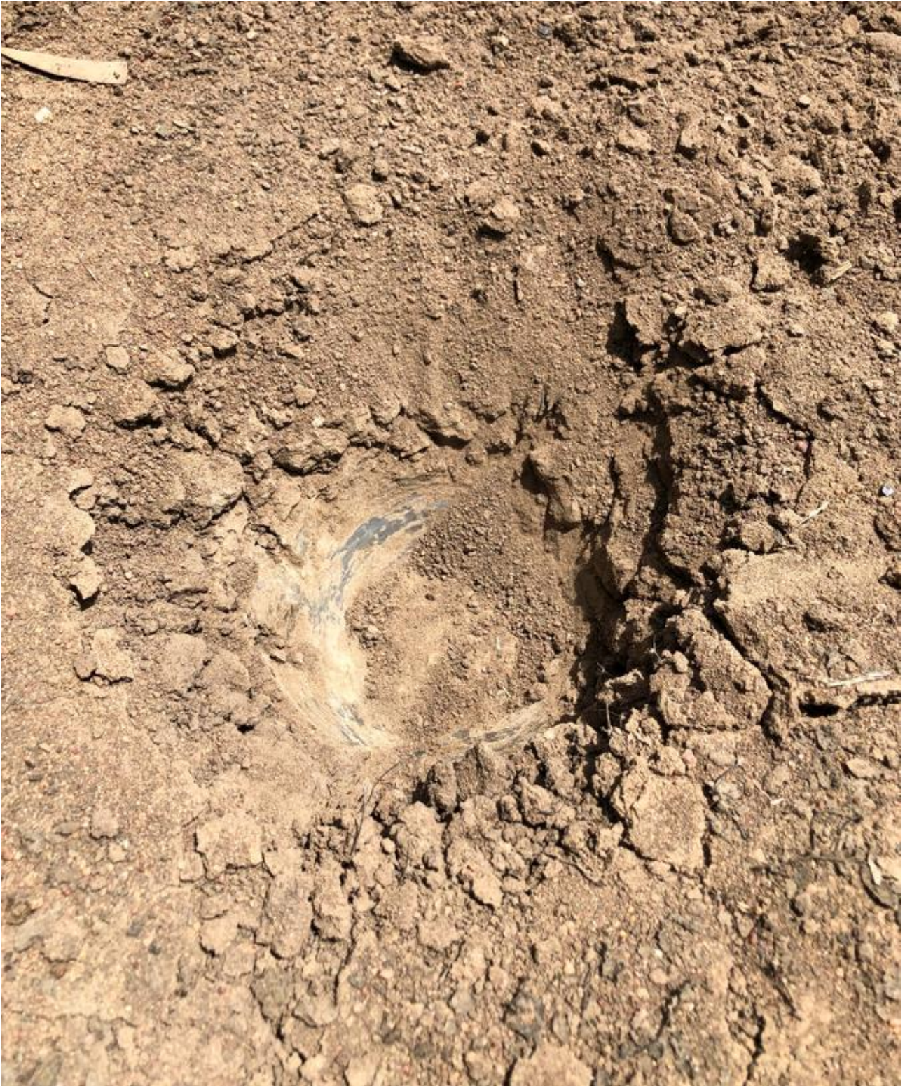
Photo 4: Attempted Hand Auger. Note compaction of clay on the bottom/edges of the bore – resulting in auger refusal
