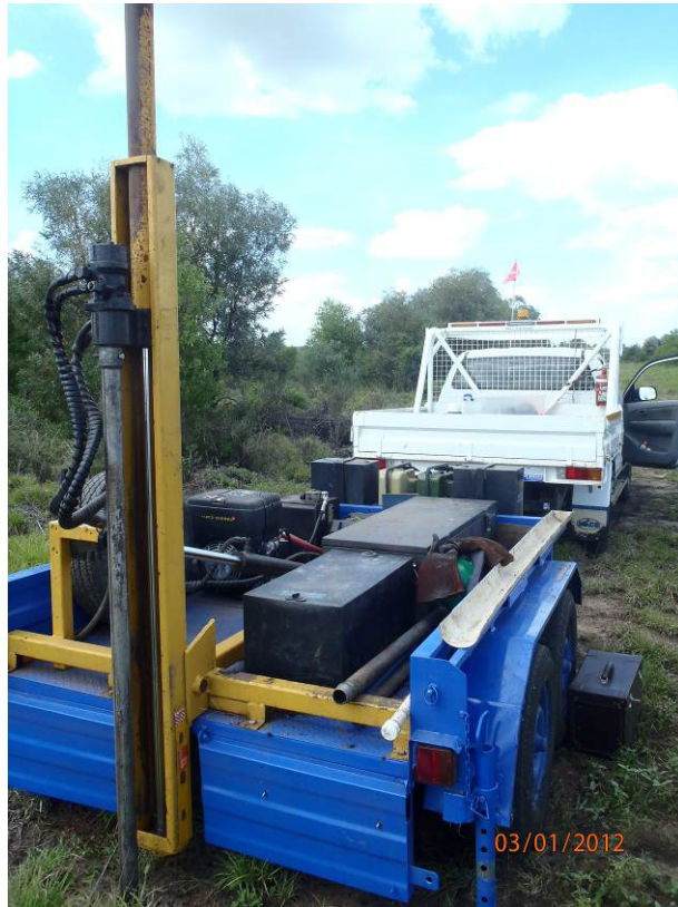
Figure 11 Coring equipment for soil sampling, Lake Vermont MLA
