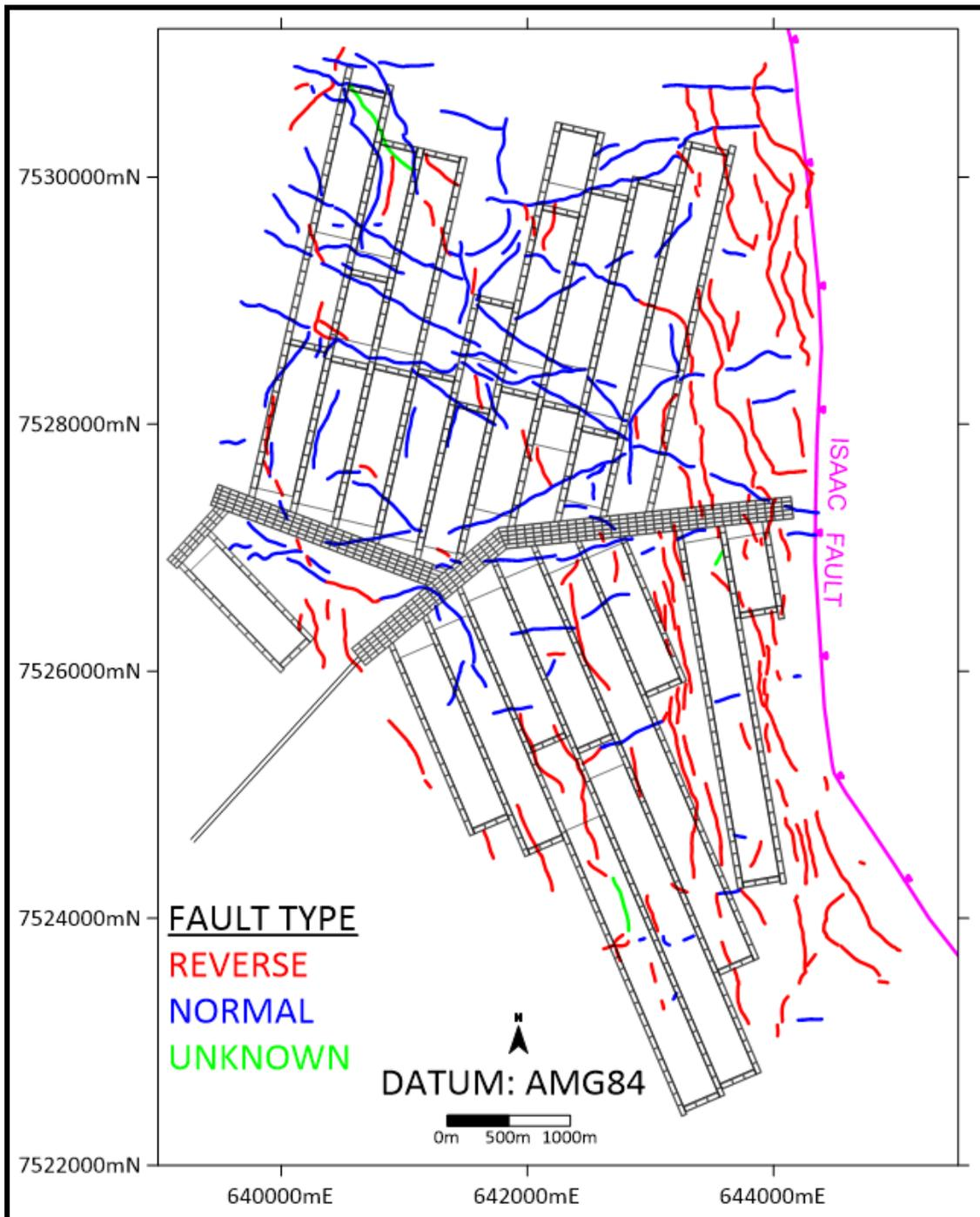
**Figure 19. Fault Types from 3D Seismic Survey – Vermont Lower Seam.**
