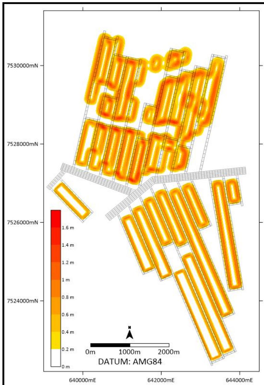
**Figure 38. Horizontal Movement after Extraction of both the LHL and VL Seams (m).**
