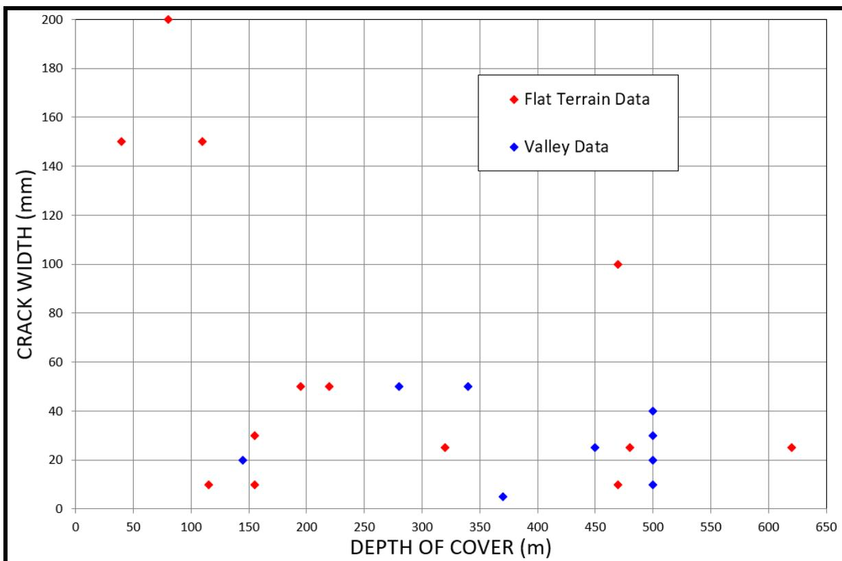
**Figure 50. Crack Width and Depth of Cover (reproduced from MSEC, 2007).**
