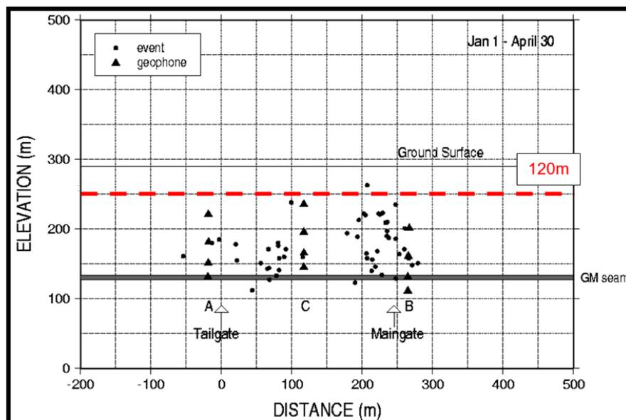
**Figure 44. Location of Microseismic Events above LW3 at the North Goonyella Mine (Kelly and Gale, 1999).**
