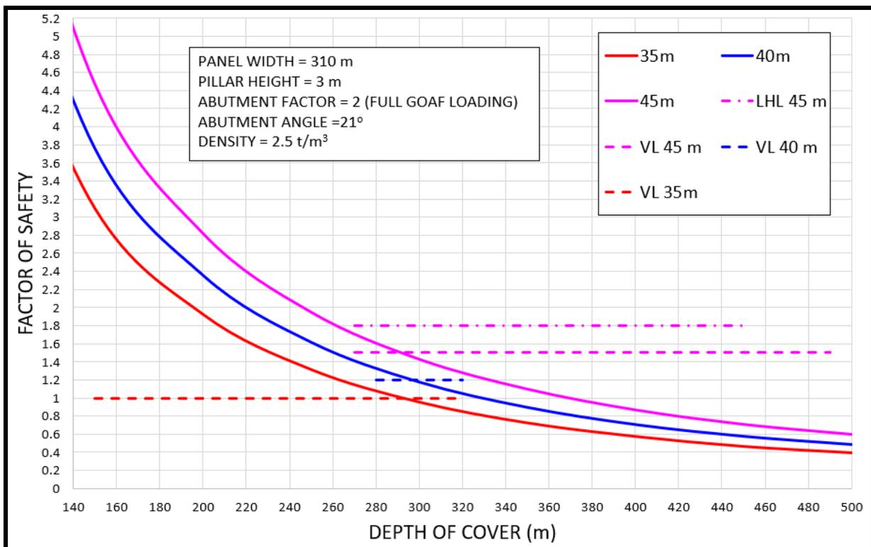
**Figure 29. Analysis of Chain Pillars using the ALPS Pillar Design Methodology.**
