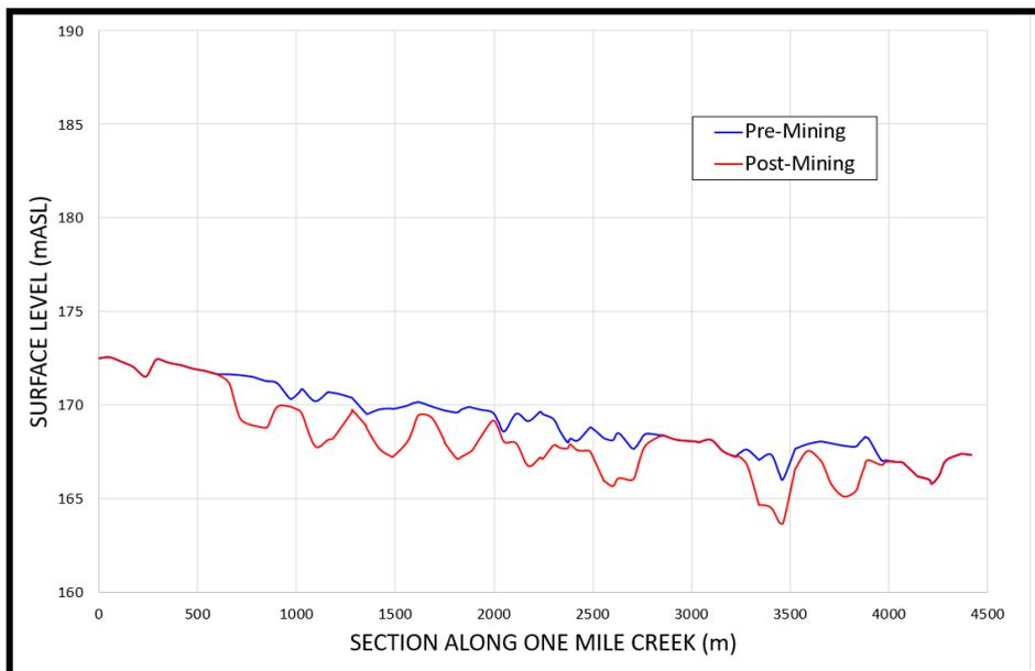
**Figure 36. Subsidence – Cross Section along One Mile Creek.**
