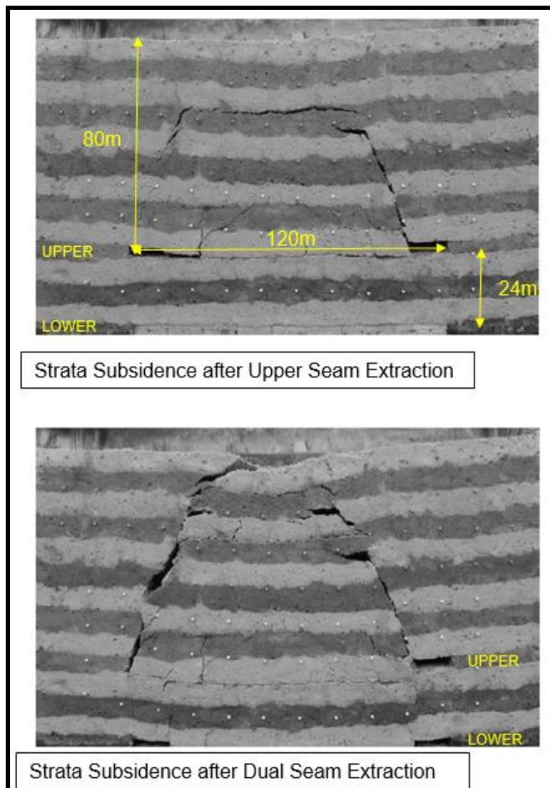
**Figure 42. Results of Physical Modelling of Dual Seam Subsidence (Ghabraie and Ren, 2014).**
