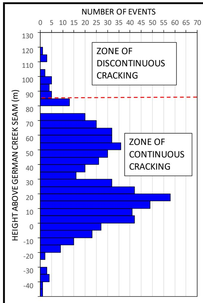
Figure 45. Location of Microseismic Events around LW101 at Kestrel Mine (Reproduced from Kelly and Gale, 1999).
