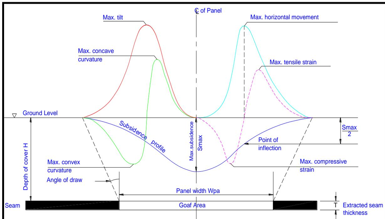
**Figure 22. General Characterisation of a Subsidence Cross Line.**
