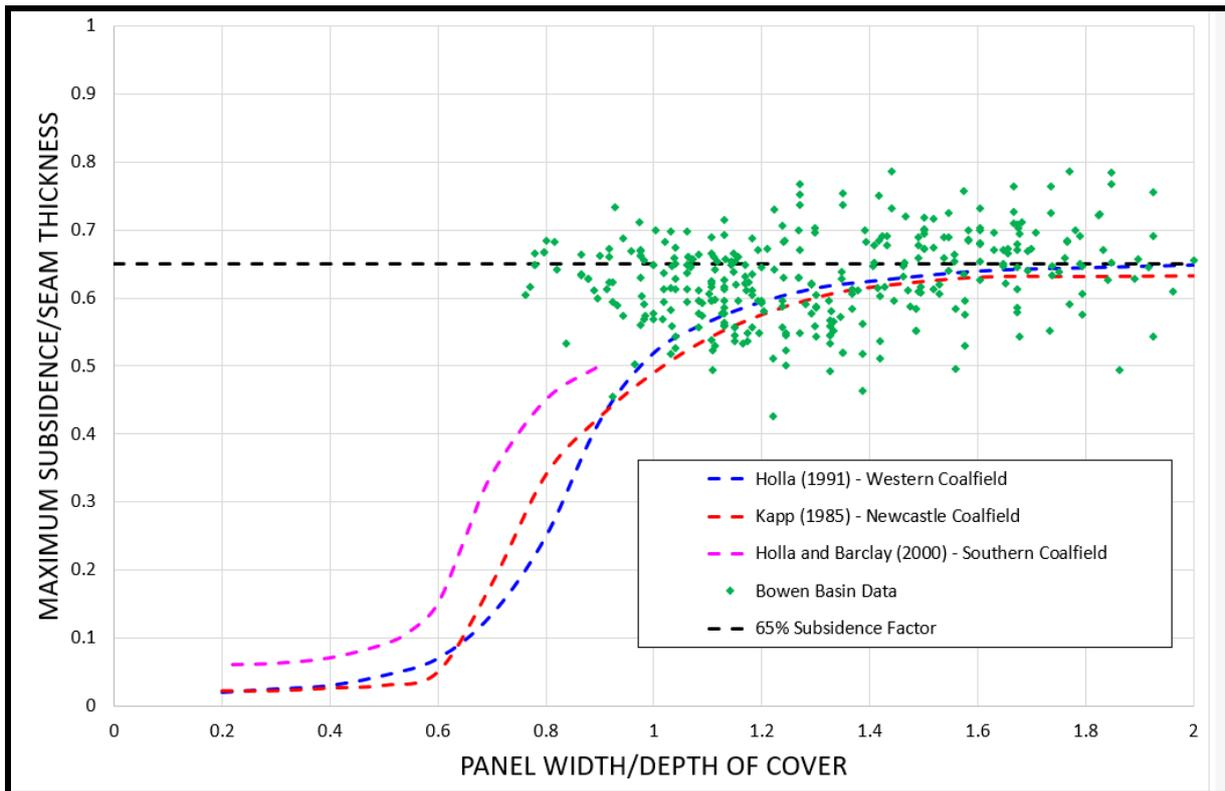
**Figure 23. Sag Subsidence over Single Longwall Panels in Virgin Ground.**
