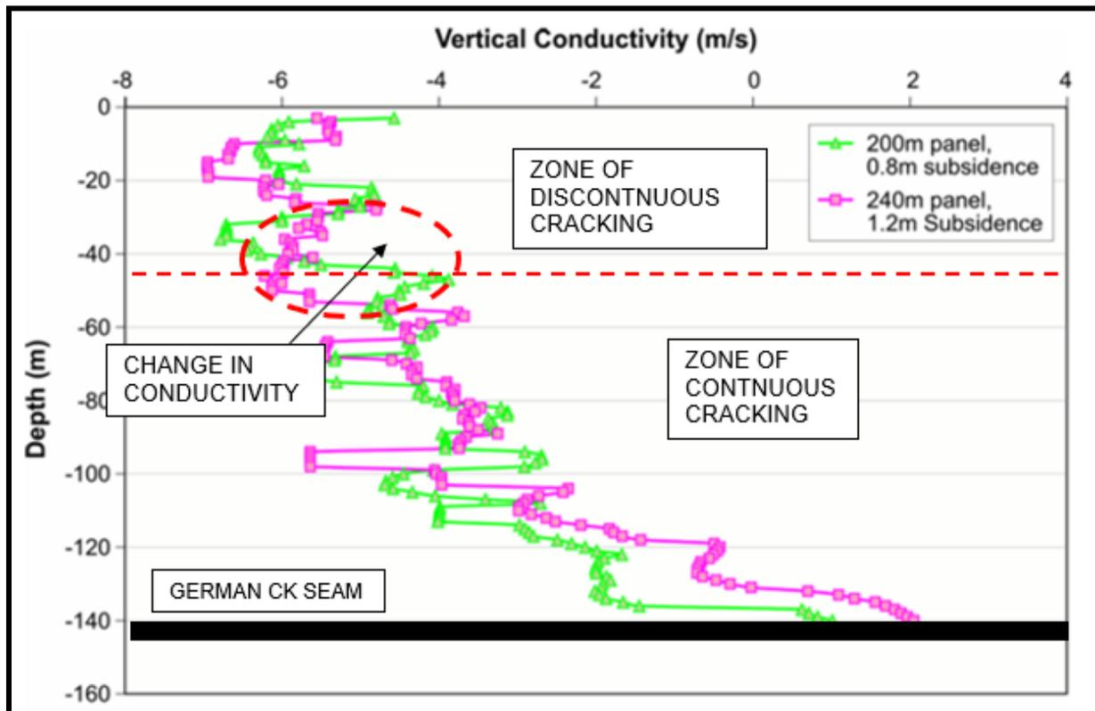
**Figure 47. Vertical Conductivity through a Numerical Model in the Southern-Oaky Creek Area (Gale, 2008).**
