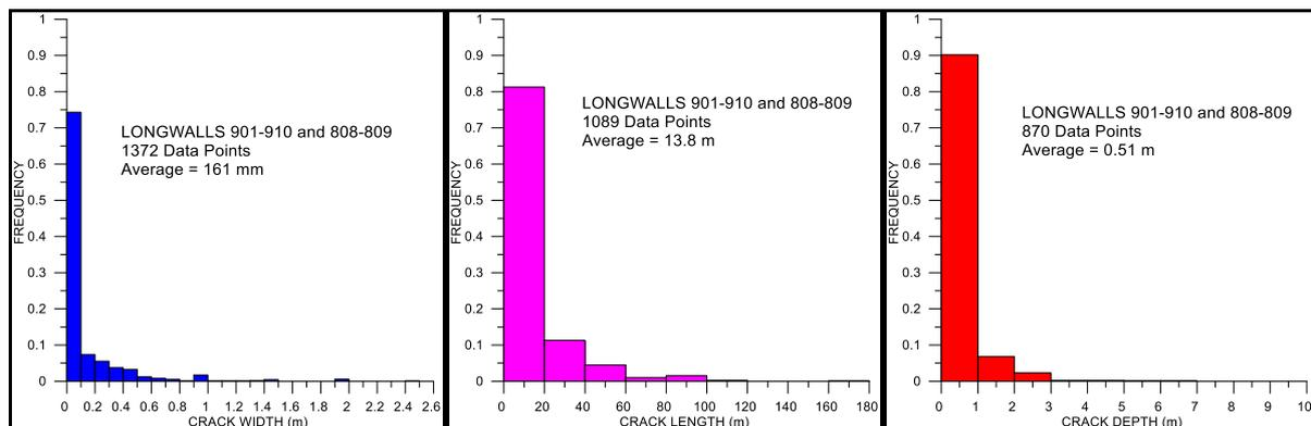
**Figure 48. Crack Data – Grasstree Mine (GGPL, 2021).**
