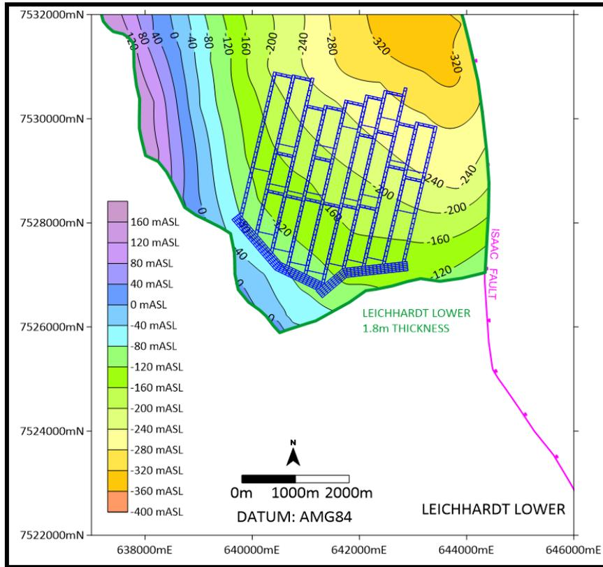
**Figure 16. Leichhardt Lower Seam Floor Levels (m ASL).**
