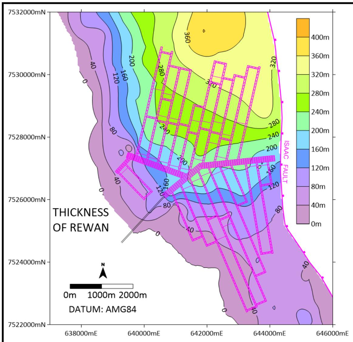
**Figure 10. Thickness of Rewan Sediments (m).**
