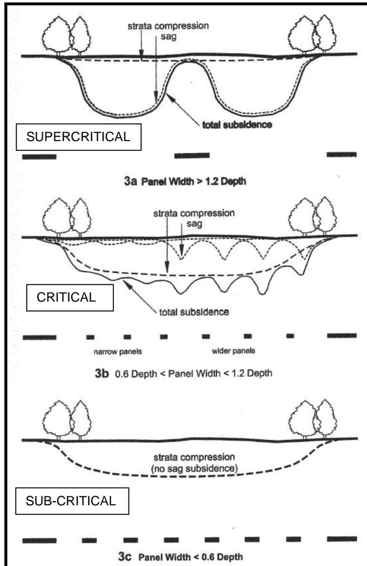
Figure 21. Effect of Panel Width (AUSIMM, 2009).
