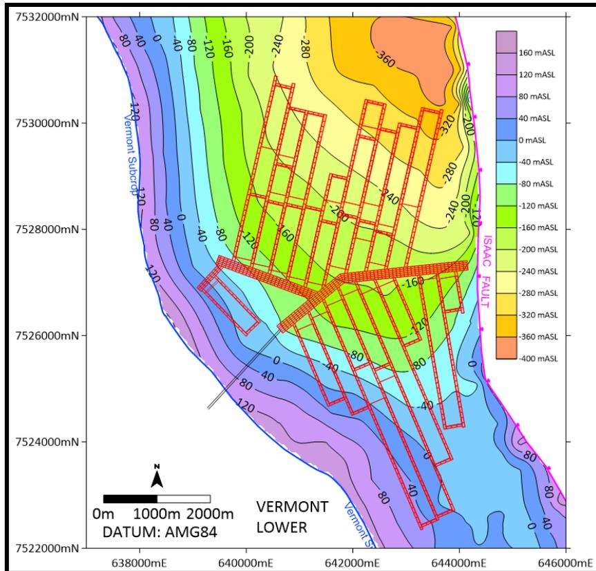
**Figure 17. Vermont Lower Seam Floor Levels (m ASL).**
