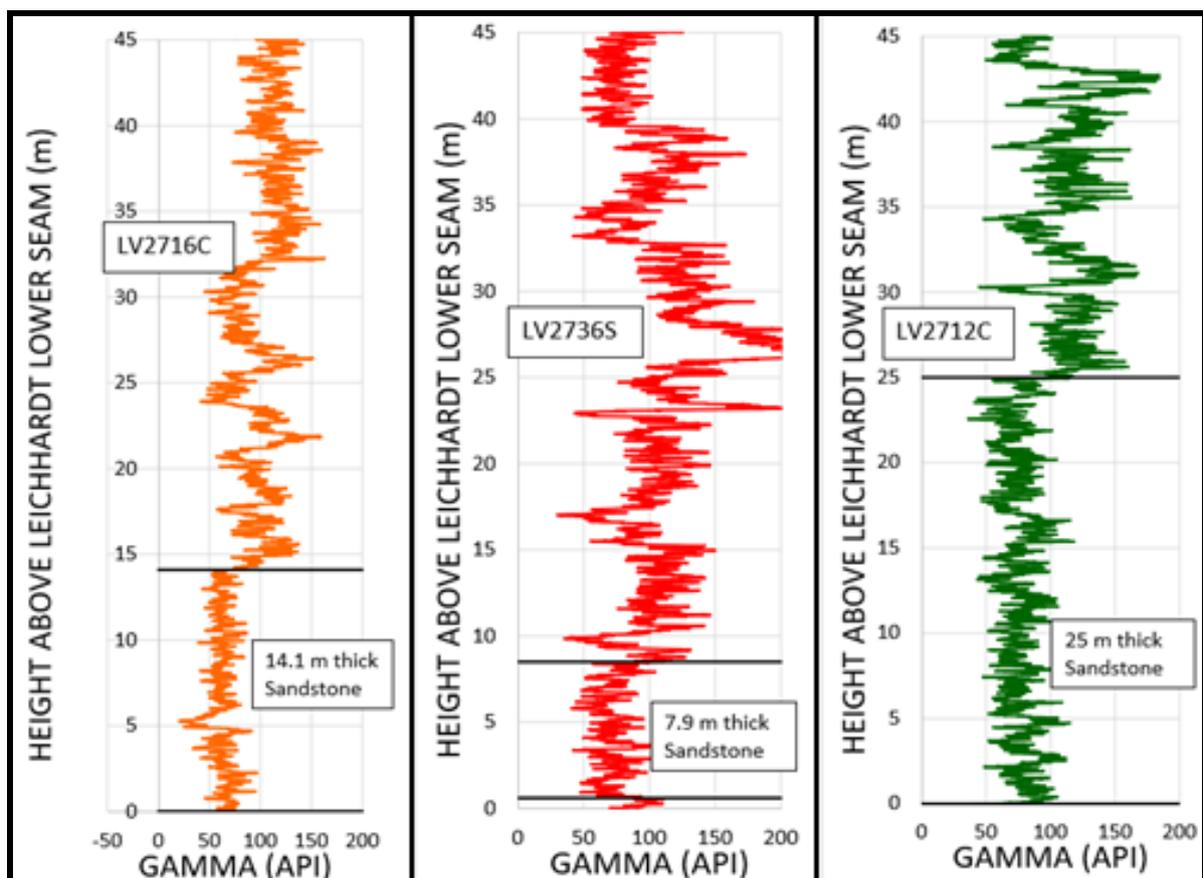
**Figure 30. Sandstone Units in the Permian above the Leichhardt Lower Seam.**
