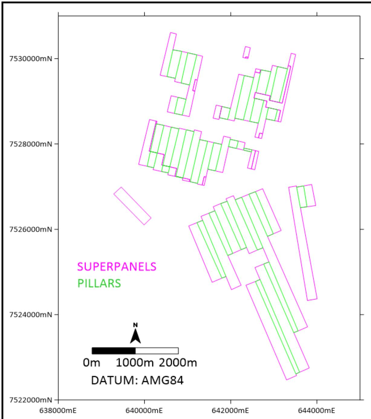
**Figure 28. Super Panels and Active Pillars with Compensated Geometries – VL Seam.**
