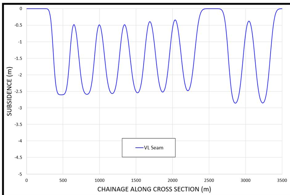
**Figure 34. Subsidence - Southern Cross Section.**
