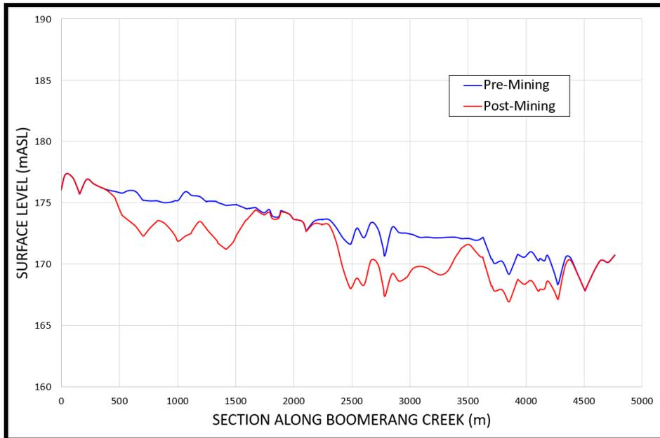
**Figure 35. Subsidence – Cross Section along Boomerang Creek.**
