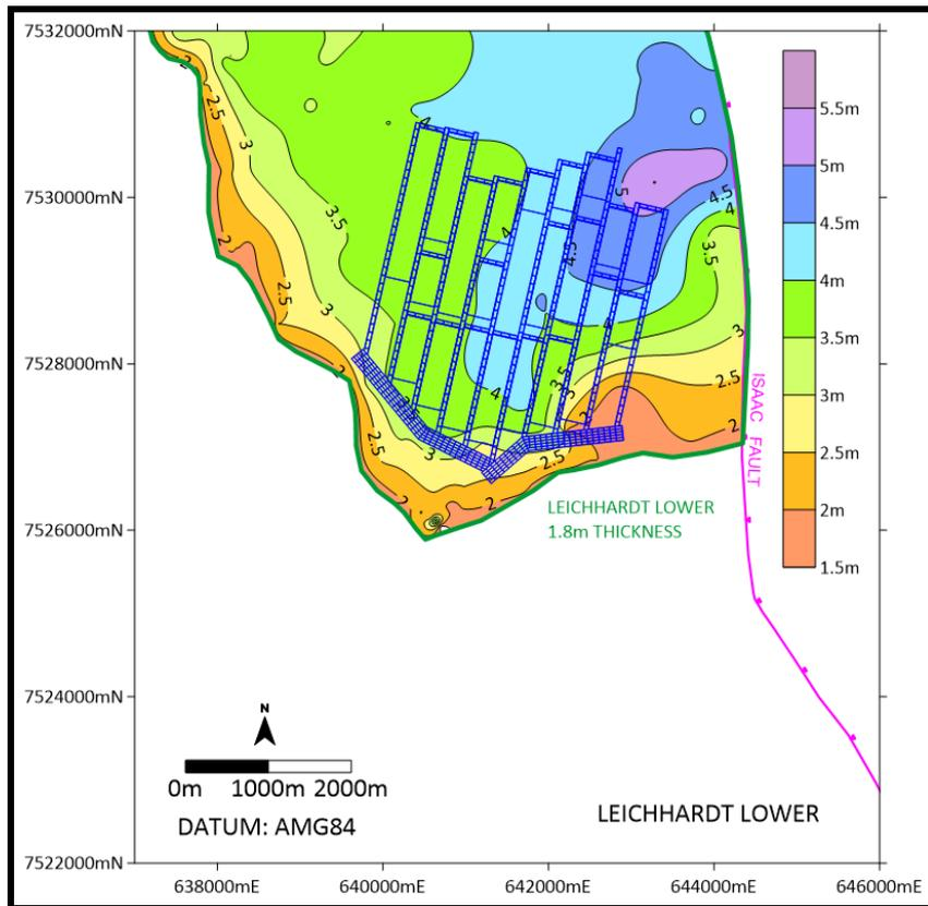
**Figure 11. Leichhardt Lower Seam Thickness (m).**
