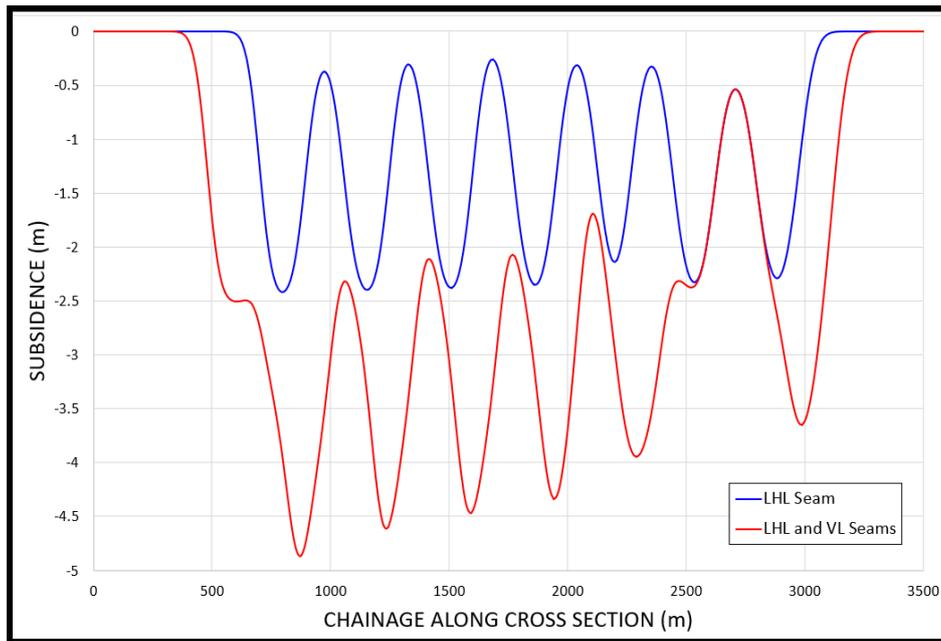
**Figure 33. Subsidence - Northern Cross Section.**
