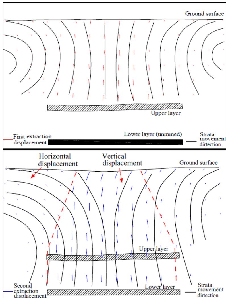
**Figure 43. Displacement Profiles of Upper and Lower Seam Extraction (Ghabraie and Ren, 2014).**
