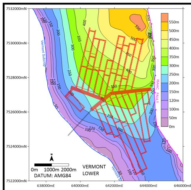
**Figure 14. Vermont Lower Seam Depth of Cover (m).**
