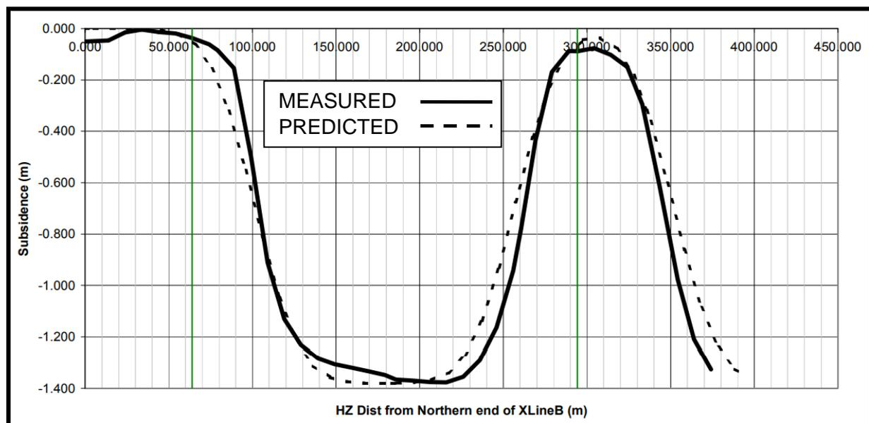
**Figure 20. Comparison of Measured versus Predicted Subsidence (Byrnes, 2003).**
