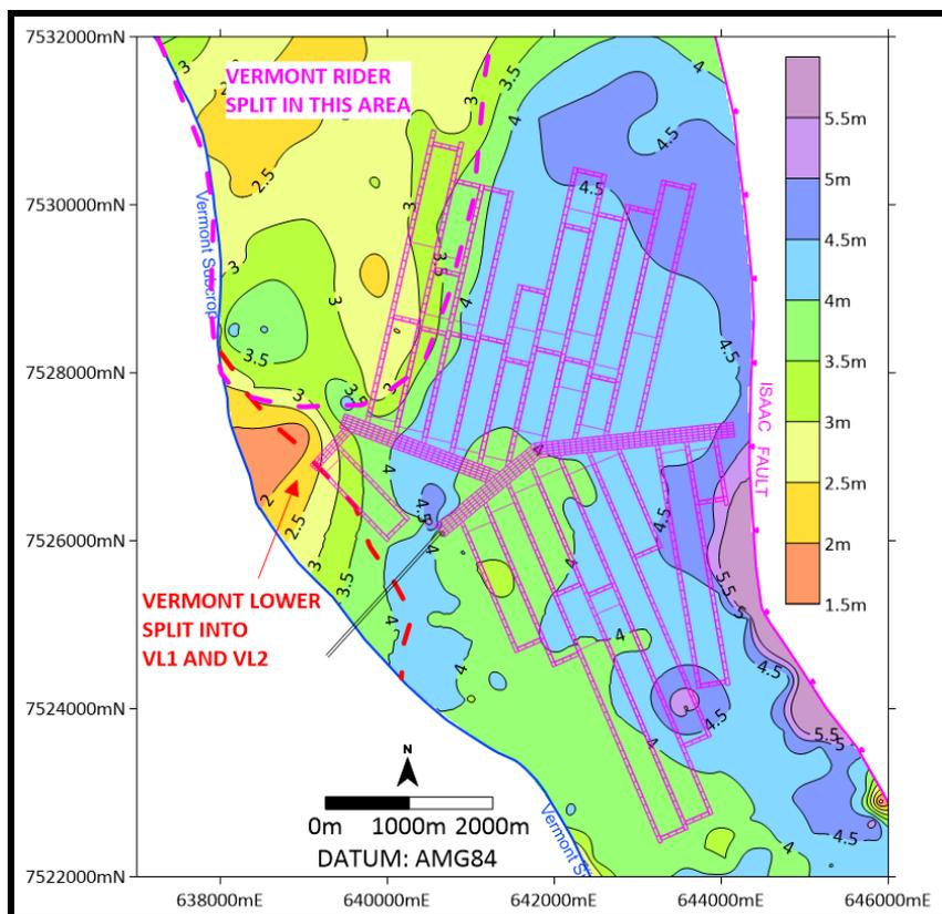
**Figure 12. Vermont Lower Seam Thickness (m).**
