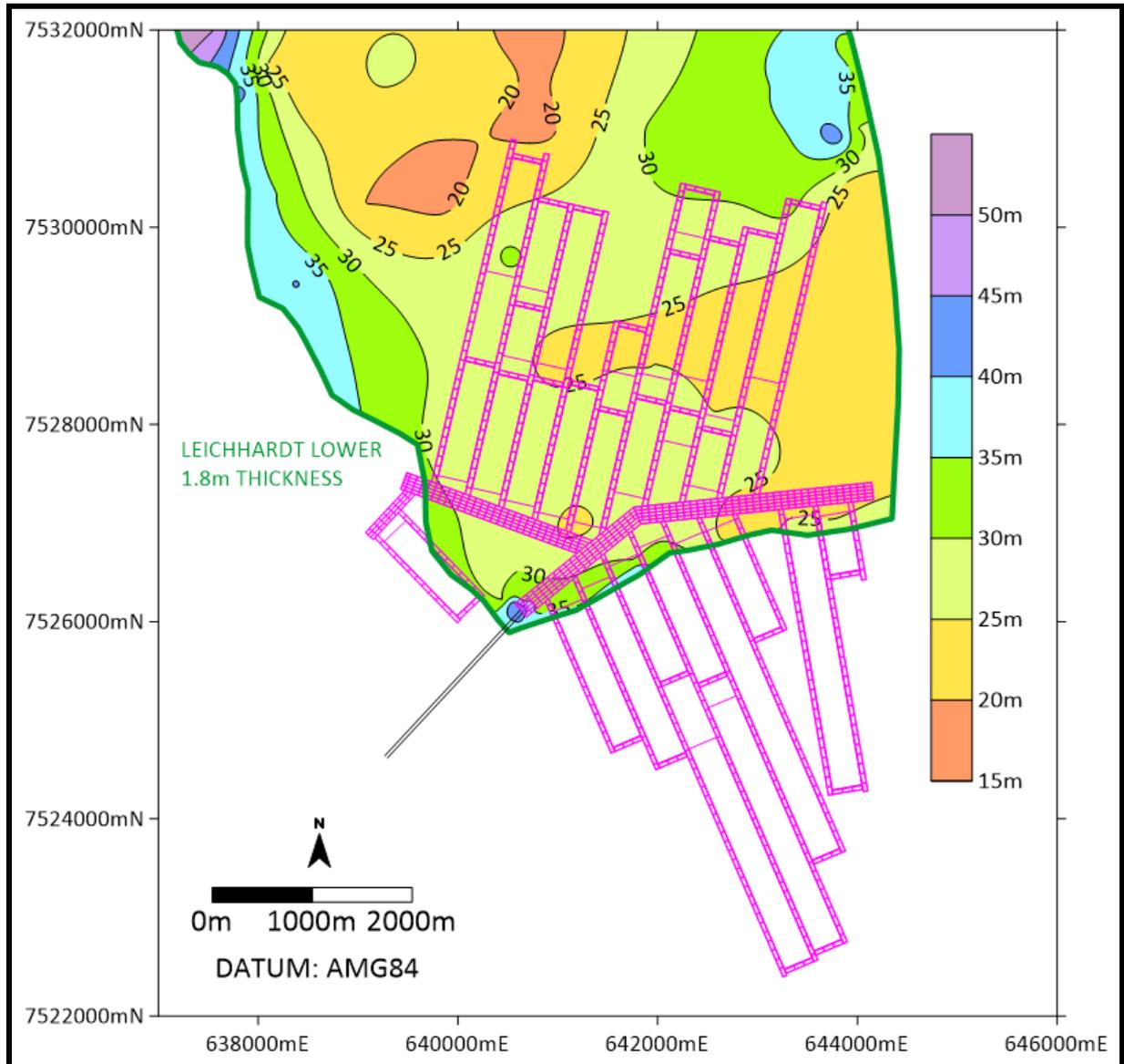
**Figure 15. Interburden Thickness between Leichhardt Lower and Vermont Lower Seams (m).**
