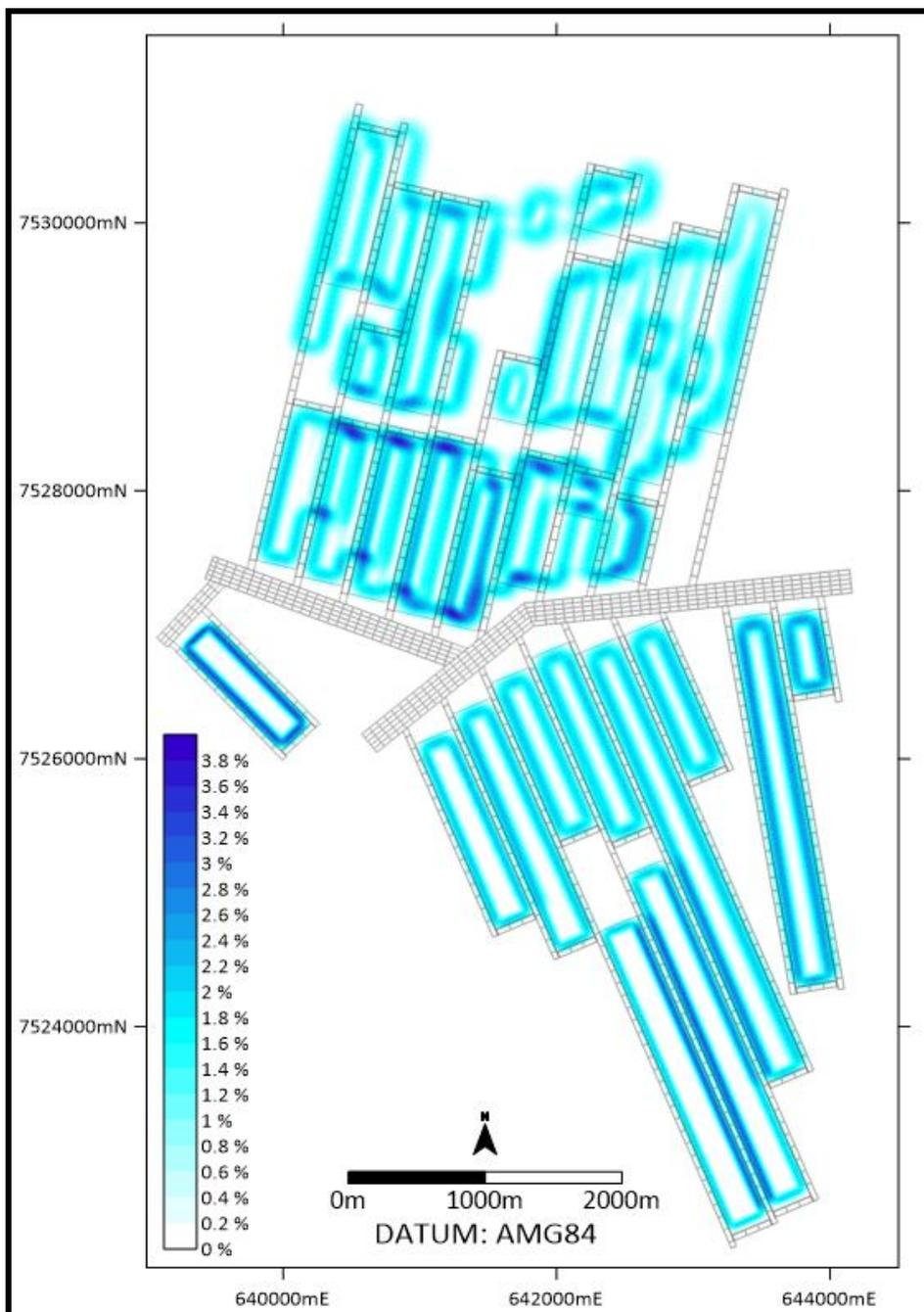
**Figure 40. Tilt after Extraction of both the LHL and VL Seams (%).**
