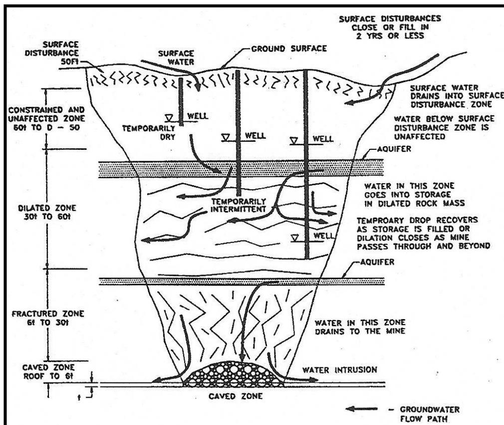
**Figure 41. Hydrogeological Model for Fracturing above Longwalls (Bai and Kendorski, 1995).**
