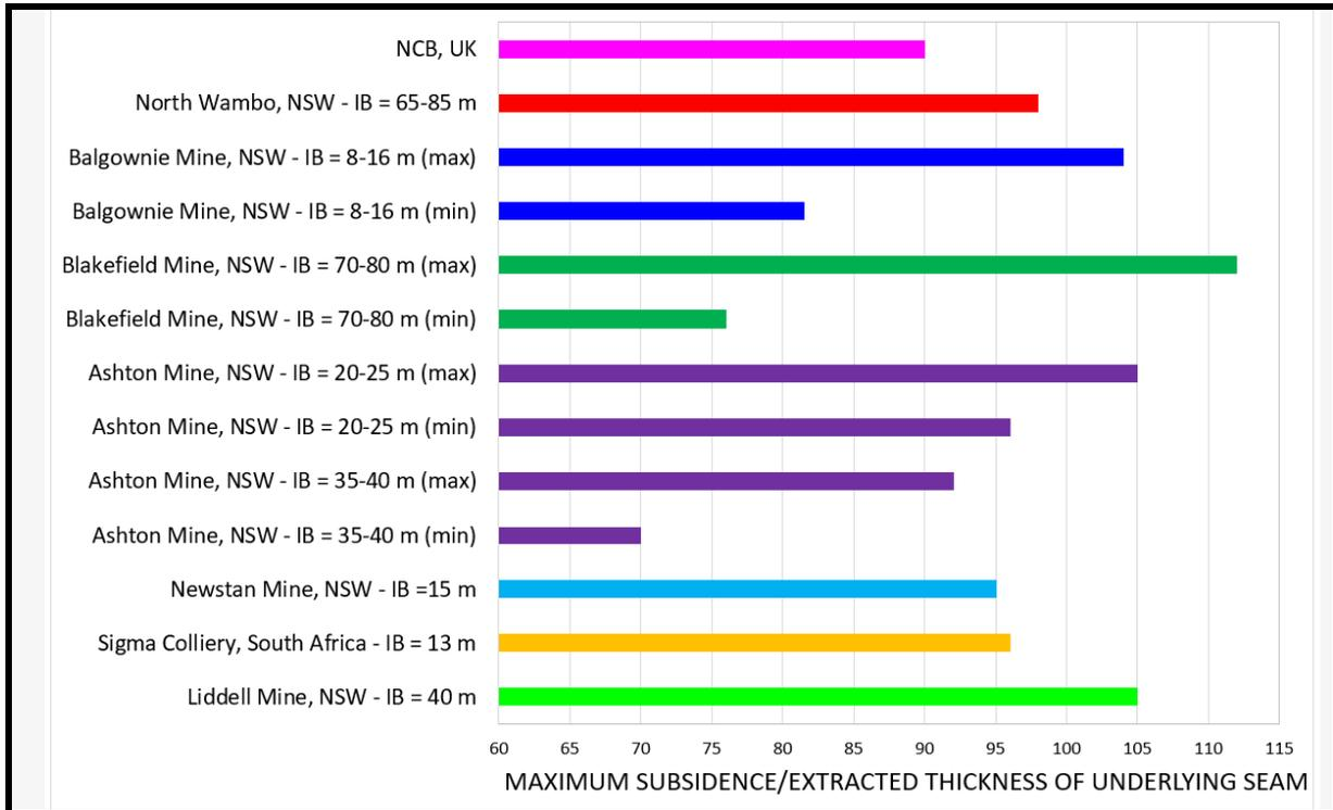
**Figure 24. Subsidence Factor for the Extraction of the Underlying Seam.**
