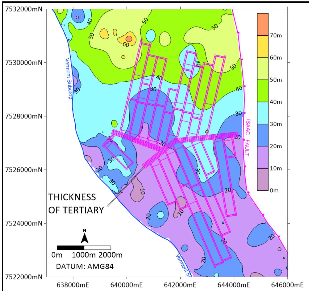
**Figure 9. Thickness of Tertiary Sediments (m).**
