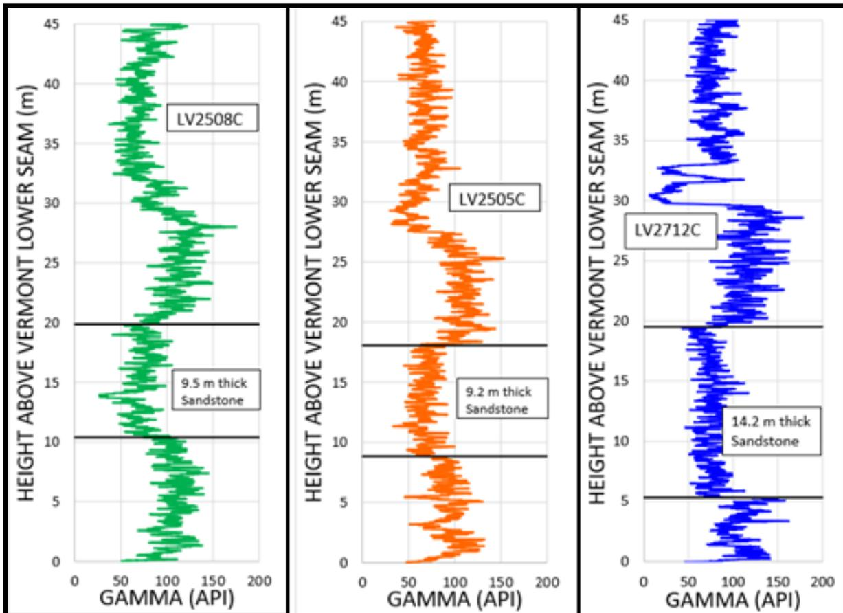
**Figure 31. Sandstone Units in the Permian above the Vermont Lower Seam.**
