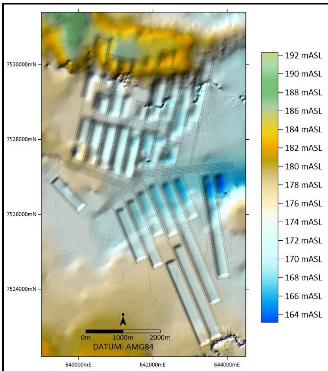
**Figure 37. Post Mining Topography after Extraction of both the LHL and VL Seams (Z=25).**
