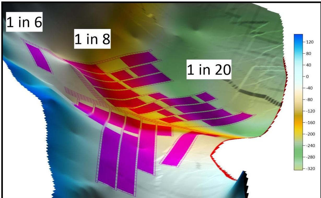
**Figure 18. 3D Surface Plot of Vermont Lower Seam Floor Levels (m ASL).**
