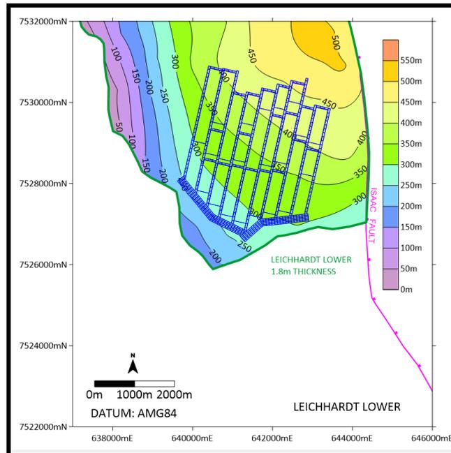
**Figure 13. Leichhardt Lower Seam Depth of Cover (m).**
