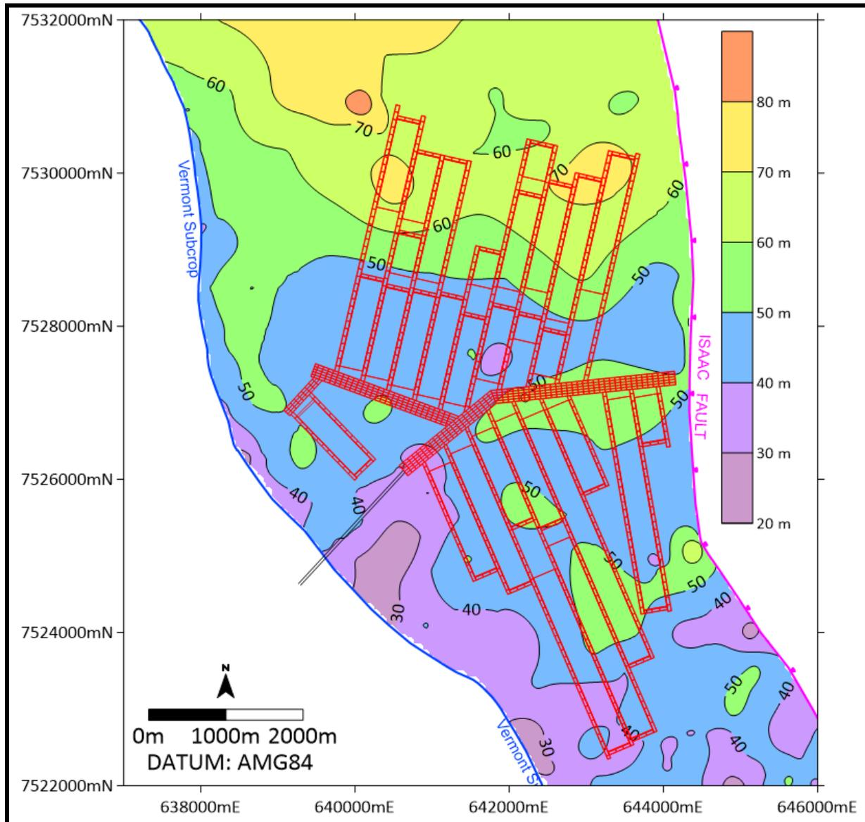
**Figure 8. Depth of Weathering (m).**
