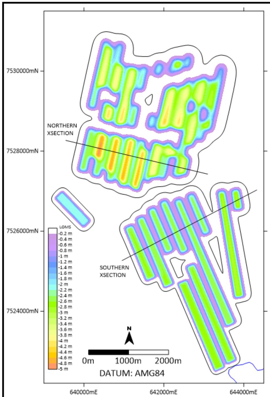
**Figure 32. Subsidence after Extraction of both the LHL and VL Seams (m).**
