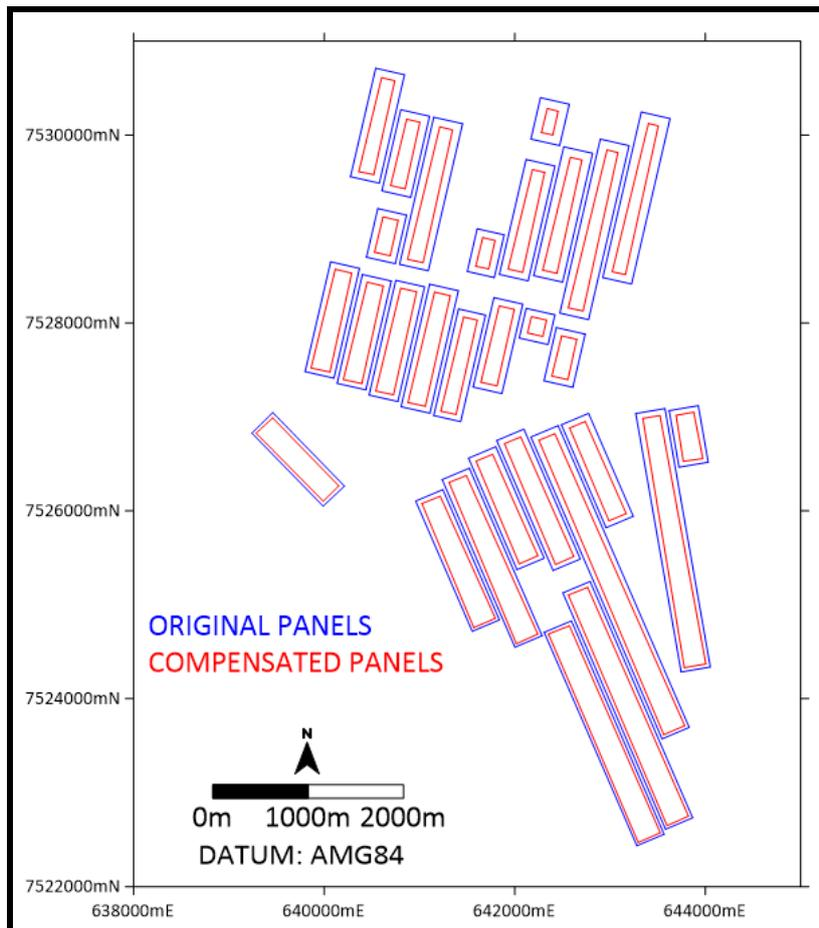
**Figure 27. Original Longwall Panels and Compensated Panels – VL Seam.**
