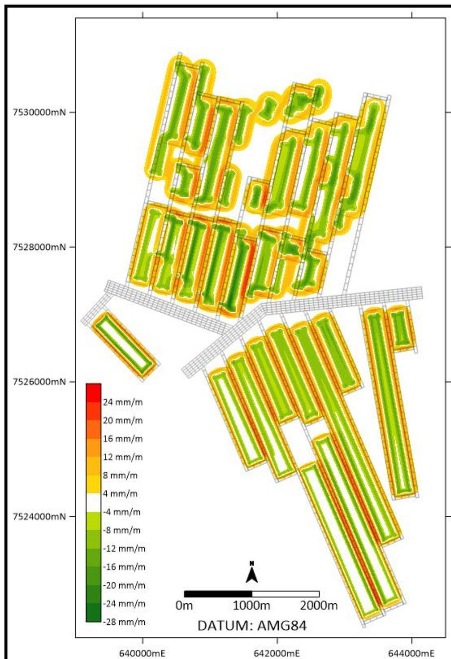
**Figure 39. Strain after Extraction of both the LHL and VL Seams (mm/m).**
