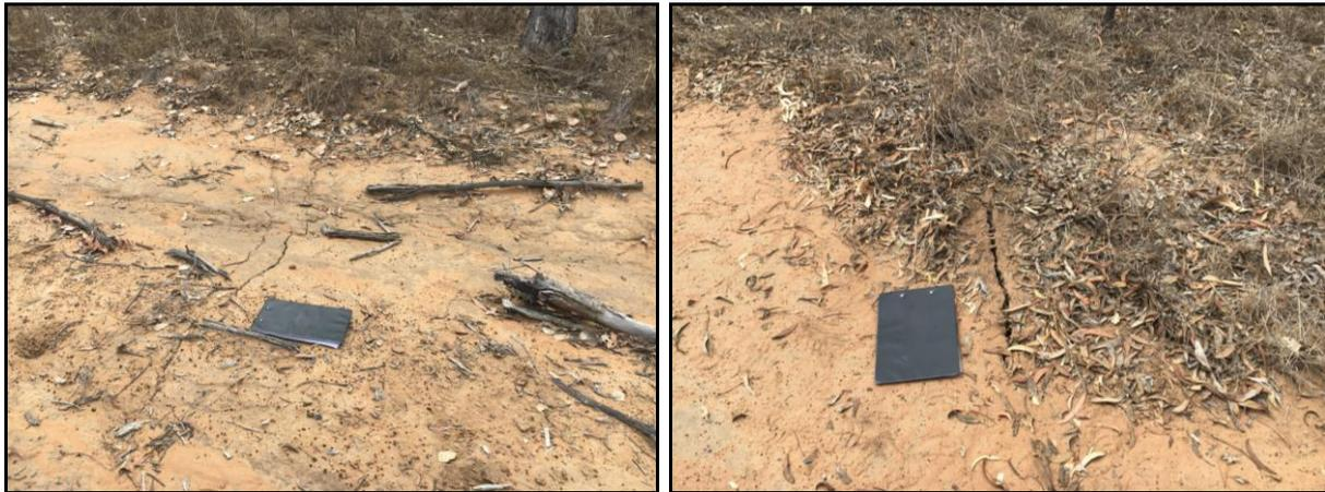
**Figure 49. Narrow Cracks at 480 m Depth of Cover – Grasstree Mine.**
